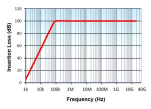
High Current Extended Performance Filters 100dB from 10kHz to 40GHz
