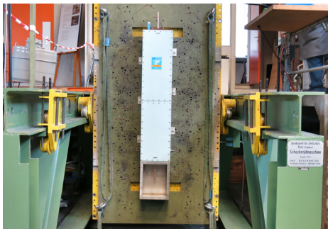
Here the vertical axis (z) of the MPE filter is being tested at the Spiez Laboratory on their large VESPA servohydraulic vertical shock tester, which can handle test objects weighing up to 10t
