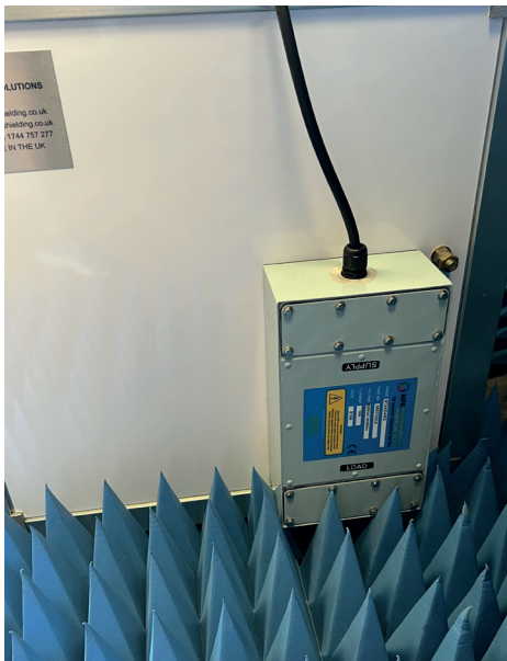
The MPE 16A high-performance power line filter, an integral part of the NTD shielded test cell
