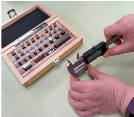
Metrology procedures at MPE include calibration with a gauge block set of the vernier caliper tool used to measure the internal and external dimensions of components
