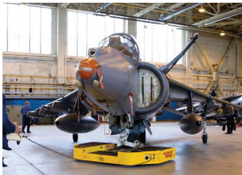
The Mantis battery-electric towing traverser from Curtiss-Wright Defense Solutions
