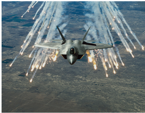
Discharge of flares to divert hostile infrared-guided missiles from target
