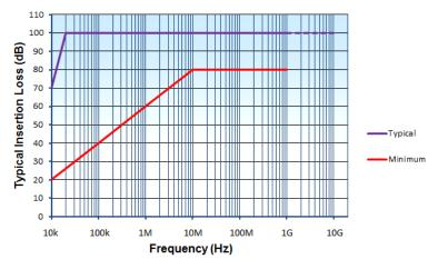
Asymmetric Performance in  $50\Omega$  System With or Without Load
