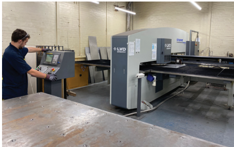
Punch press operation at MPE on the high-performance LVD Strippit
