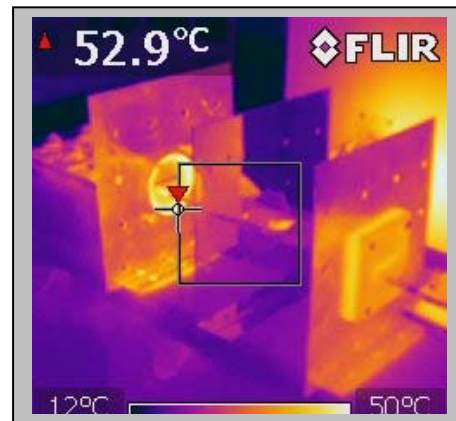
Figure 2. Eddy Current Heating in Steel Barriers
