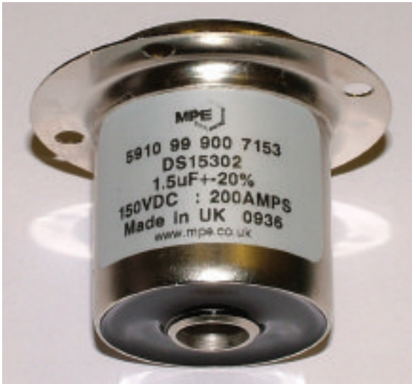
MPE feedthrough capacitors (such as the model DS15302 shown) are designed for through-bulkhead mounting to provide high-frequency EMC filtering in line-to-ground applications
