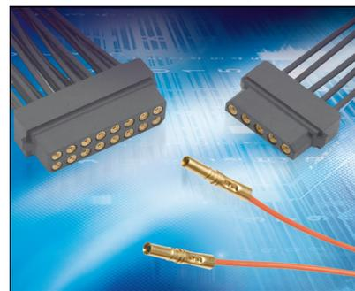
32AWG wire. It provides a current rating of 3.3A in isolation and 3A on all contacts simultaneously. The crimp contact is gold plated. It has a contact resistance of 25mΩ and operates at temperatures between -55 and +125°C. The crimp contact is suitable for use in robotics,
