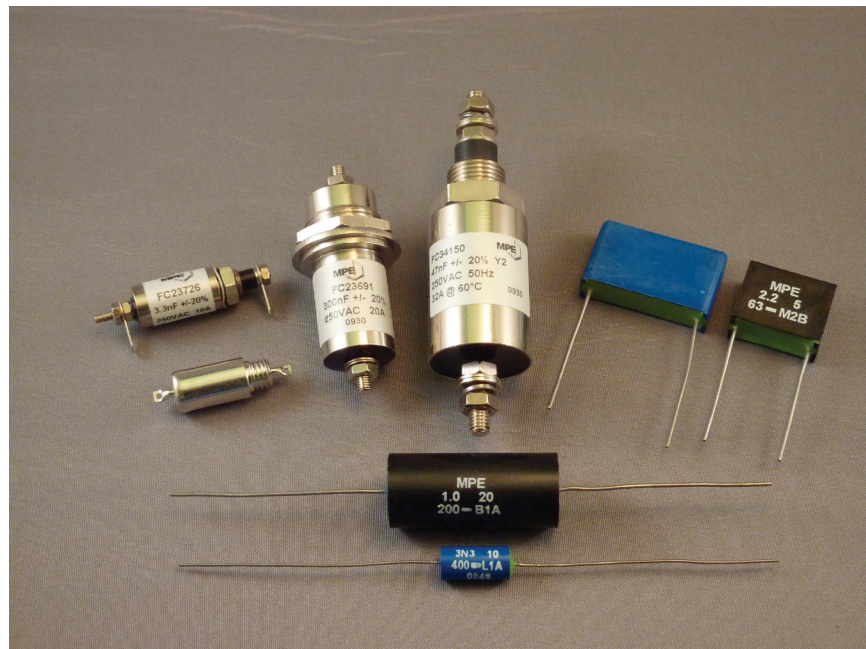
Figure 2: Typical feedthrough capacitors compared with two-terminal capacitors
