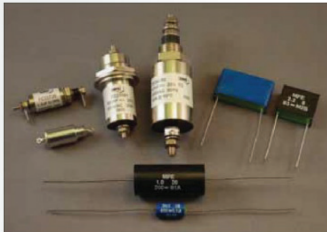
Figure 2. Typical feedthrough capacitors compared with two-terminal capacitors.
