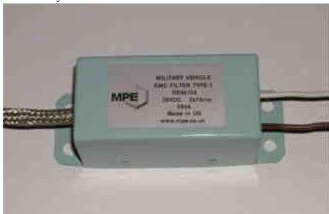
Many items of equipment in military vehicles such as blower or wiper motors need filtering at frequencies beyond 1GHz, and it is not always practical to fit filters through a bulkhead or mount equipment inside a shielded enclosure. A standard solution is to use a filter with integral screened cables which shield the "dirty" cables emerging from the equipment, to prevent the cables radiating until the noise has been safely removed by the filter.
