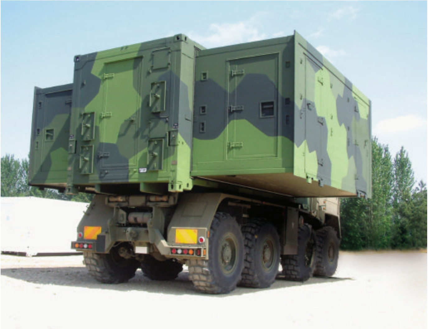
Another example of a vehicle-mounted tactical mobile communications system shelter with side extensions deployed
