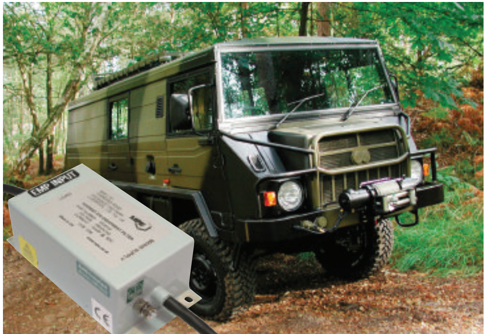
C4ISTAR equipment can also be vehicle-mounted, like this Cormorant communications system developed for the British Army. INSET: a close-up of one of the MPE filters used in this installation
