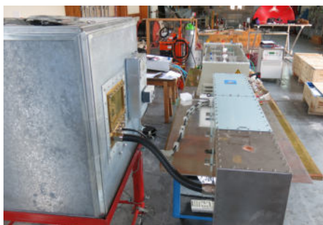
Shock testing of MPE HEMP filter in the Spiez Laboratory
