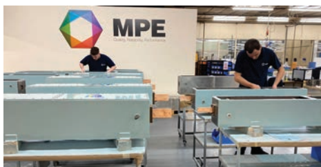
A batch of large high-current HEMP protection filters in final assembly at MPE
