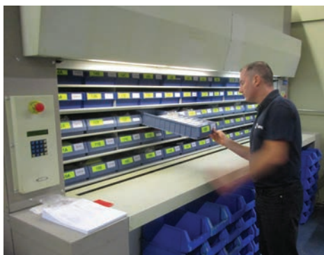
An operator can access a component from the drawer of the automated carousel a few seconds after entering the required part number via the keypad on the left
