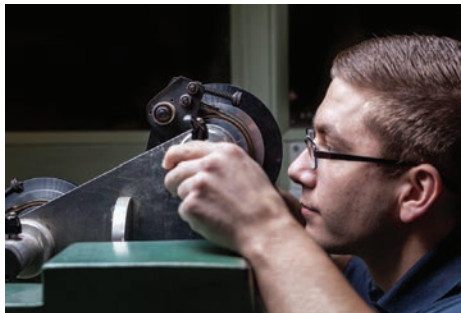
Kieron Campbell inspects capacitor winding with metallised plastic film
