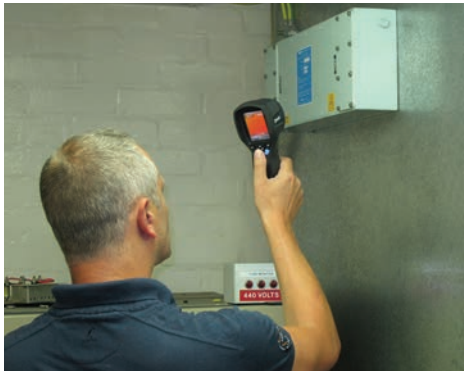
An MPE engineer uses thermal imaging to check a filter under test
