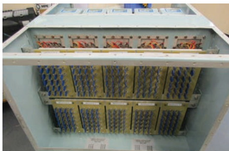
The largest ever single order for telephone line filters in MPE's history – a 240-line unit, 10 modules of 24 lines each, with varistor PCBs fitted
