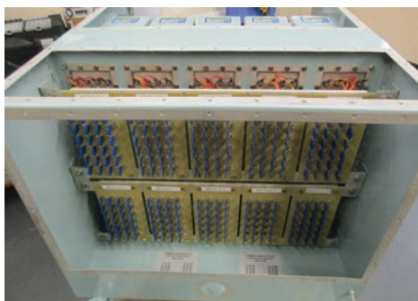
A 240-line unit (10 modules of 24 lines each) with varistor PCBs fitted
