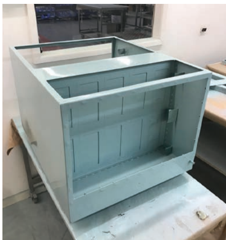
The outer steel enclosure during MPE's in-house paint spray process
