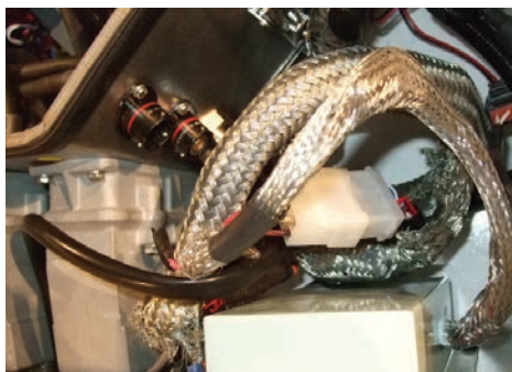
A typical configuration often tested – an MPE EMC filter with shielded cables in close proximity to each other, shown here in the power compartment of a defence aerospace application. Mechanically, pre-compliance testing work can also highlight the very tight space constraints that may apply to housing a filter product.
