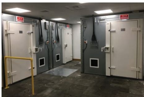
NTD Shielding Services application of custom-designed RFI shielded chambers. Each houses a comprehensive electrical wiring system with incoming power lines located behind a pneumatic door as pictured here.
