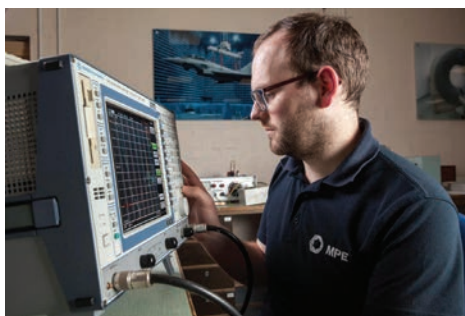
Electronic testing of filter performance with oscilloscope at MPE
