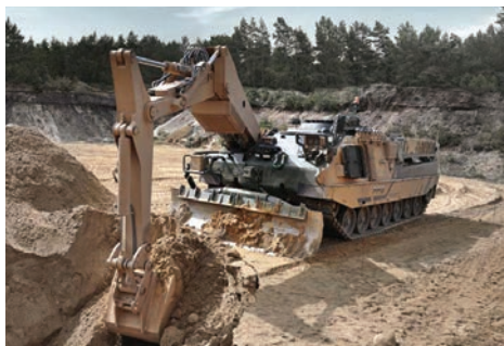
WISENT 2 operating in its armoured engineer vehicle configuration
