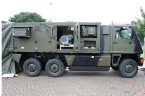
A Marshall ADG GEOINT shelter for the British Army as mounted onto a MOWAG Duro 6x6 all-terrain tactical military vehicle
