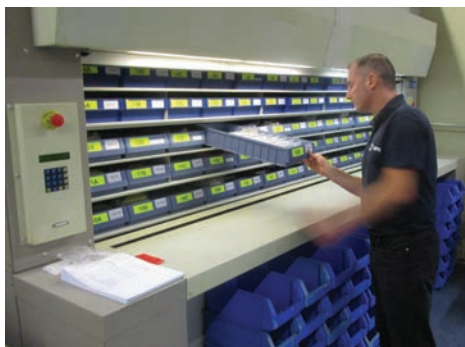
The new automated storage carousel at MPE enables an operator to access required parts in seconds
