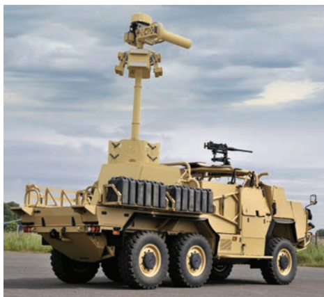
In this typical application, Nordic Defence & Security supplied the telescopic mounting structure for the new Coyote anti-UAV tactical support vehicle designed and built by the British special operations vehicle developer Supacat
