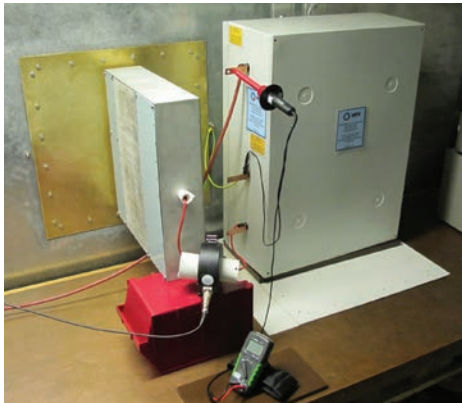
The Marx pulse generator installed within MPE's in-house screened room test facility
