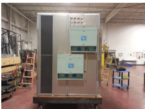
MPE filters mounted to shield for shield effectiveness testing at DeTech, Virginia
