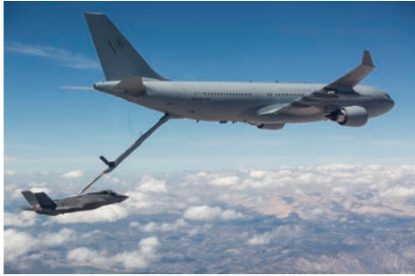
Air-to-air refuelling by an Airbus A330 tanker of the Royal Australian Air Force (RAAF)
