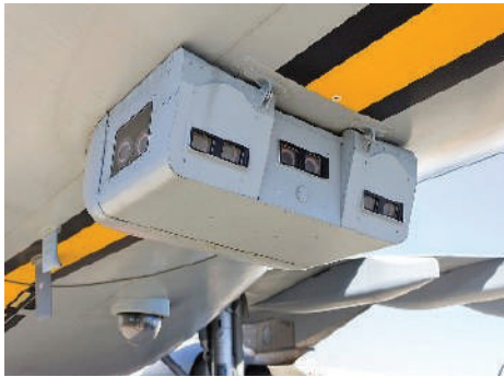
A Kappa Enhanced Vision System camera as mounted on the A330 refuelling tanker for in-flight surveillance
