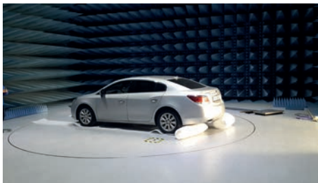
Anechoic chamber installation by Eretec for automotive testing at the INFAC Corporation in Korea
