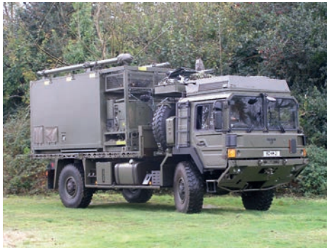
Falcon system mounted on the British Army's MAN 4x4, 6-tonne, HX60 truck
