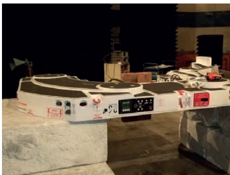
Pre-compliance EMC testing of the Mantis towing traverser
