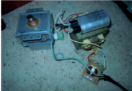
Figure 2 - Microwave oven as an IEMI source (image by courtesy of QinetiQ)
