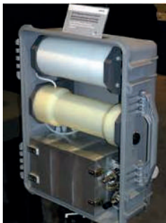
Figure 3 - Diehl briefcase mesoband UWB source
