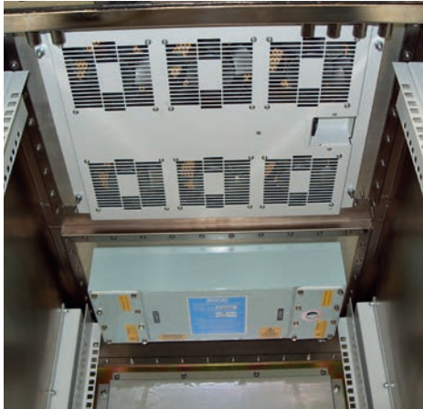
A Barton Engineering TEMPEST rack with 10A MPE filter for filtering the electrical cable entering the cabinet
