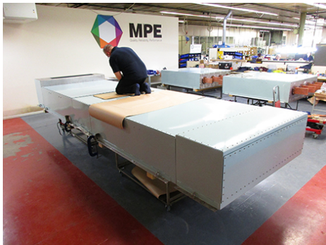
A custom MPE 3000A very high current (VHC) EMP power line filter with TEMPEST performance
